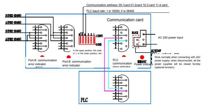
Liyuan Rectifier RS 485 Network Control System is a digital, effective, rapid and stable communication system. It consists of a master machine, PLC, LY-RS232/RS485 and a slave machine (a rectifier equipped with a network control card RS485.
