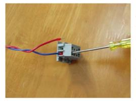
Communication terminal for rectifier, refer to diagram, first use little flat-head screwdriver to insert into small hole of terminal top, then make screwdriver to vertically force into such hole along terminal until side face of terminal has small hole to open enough to insert communication conduction wire (or that with insertion pin), at last pull it out by force till conduction wire fails to pull out; as for terminal for terminal, refer to (3), it only needs one group of wire.
