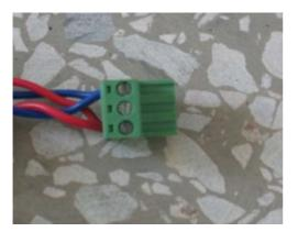
Communication terminal for control terminal, refer to drawing, first peel two sets of communication A wire for some distance, and then twist it together, and then use flat-head screwdriver to operate it under method specified above, and clip A line into it, connection with B line is same as that of A. After connection, operator must pull it out by force once, so as to that communication line is hard to be pulled out from terminal.
