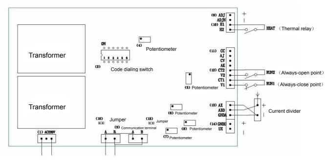
(1) AC220V power input terminal, all specified power are 15W, 50HZ (60HZ) , it is recommend to use not less than 0.5mm<sup>2</sup> power section area.
