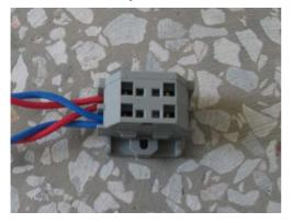
Communication terminal for rectifier, refer to drawing, first peel two sets of communication A wire for some distance, and then twist it together, and then use flat-head screwdriver to operate it under method specified above, and clip A line into it, connection with B line is same as that of A. After connection, operator must pull it out by force once, so as to that communication line is hard to be pulled out from terminal.
